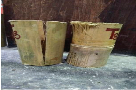
FIGURE 5. Shear strength test: Internode and node
