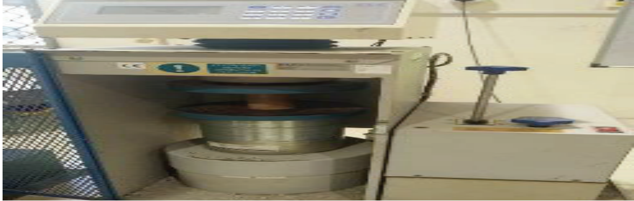
FIGURE 1. Setup for compression test
